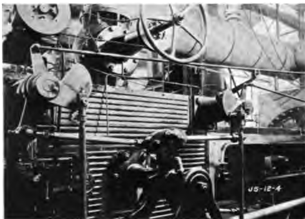
Fig. 3. Guards for Shear-Points in Hooks of Corliss Valve Gear. Fig. 4. Hooks of Corliss Valve Gear with Guards removed.†
